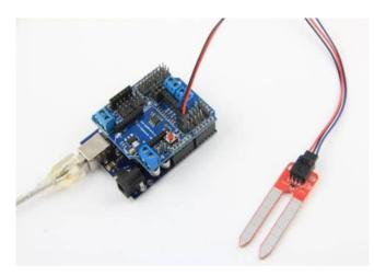
Figure 2: Soil Moisture Sensor Compatible with Microcontroller
