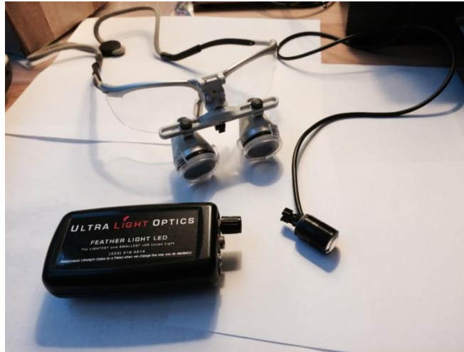
Figure 1: Completed OraLite system integrated with dental optics
