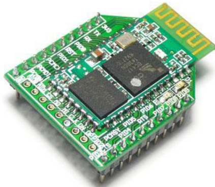
Figure 9: Bluetooth Bee Master Module
