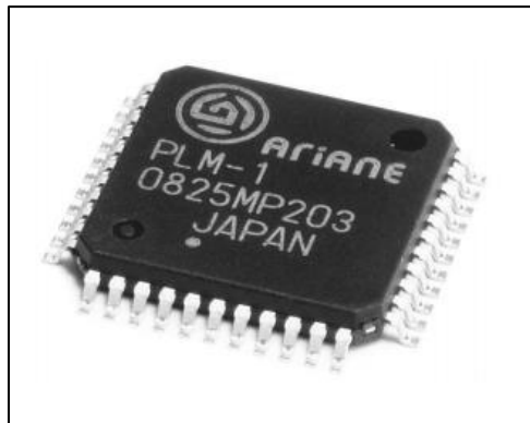
Figure 5: PLM-1 power-line modem from Ariane Controls
