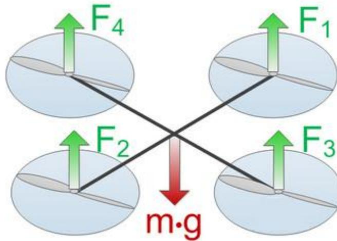
**Figure 7:** Balance of forces due to the motors and gravity. [5]
