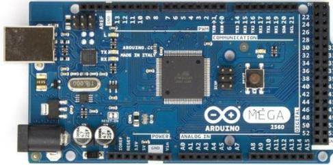
**Figure 5:** The Arduino Mega 2560. [10]
