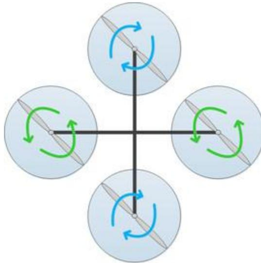
**Figure 4:** The rotation of the corresponding opposite motors. [5]
