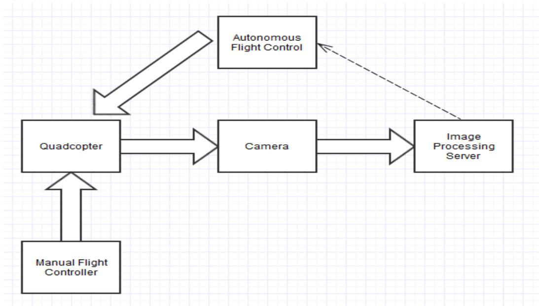
**Figure 1:** The SearcUE system consisting of its fundamental components and their relations.
