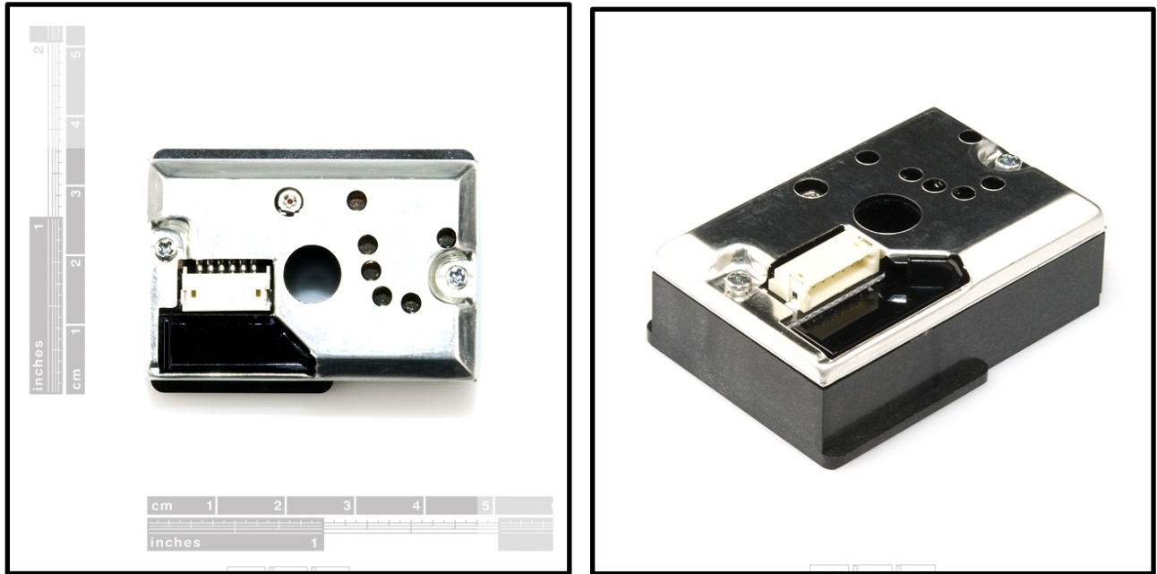
Figure 9: Top and diagonal view of Sharp ODS [4]
