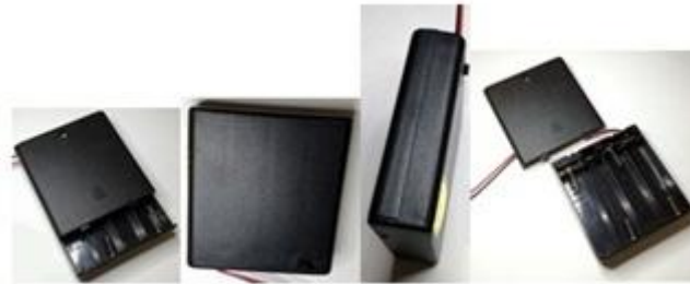
FIGURE 24: 6V BATTERY PACK FOR THE LED'S AND MOTORS
