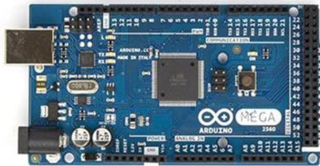
FIGURE 7: ARDUINO MEGA 2560 - ATMEGA 2560 MICROPROCESSOR
