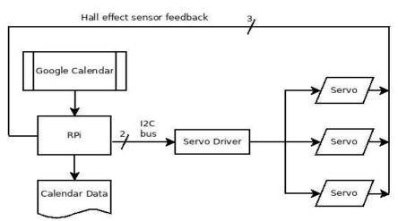
Figure 8: Controller block diagram with Hall Effect feedback
