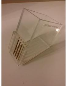
Figure 6: Hopper assembly after laser cutting
