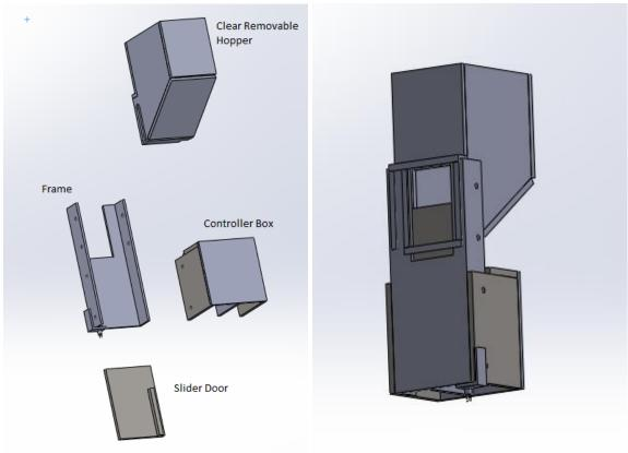
Figure 1: Four parts of AutoFeed
