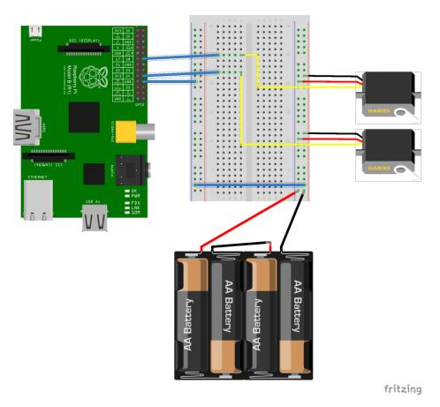
Figure 7: HS-422 servo motor test circuit
