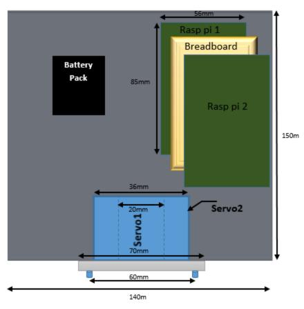
Figure 11: 2D sketch of 3 floor design (Design2)
