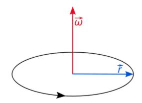
Figure 20: Definition of positive rotation reported by a gyroscope [23]
