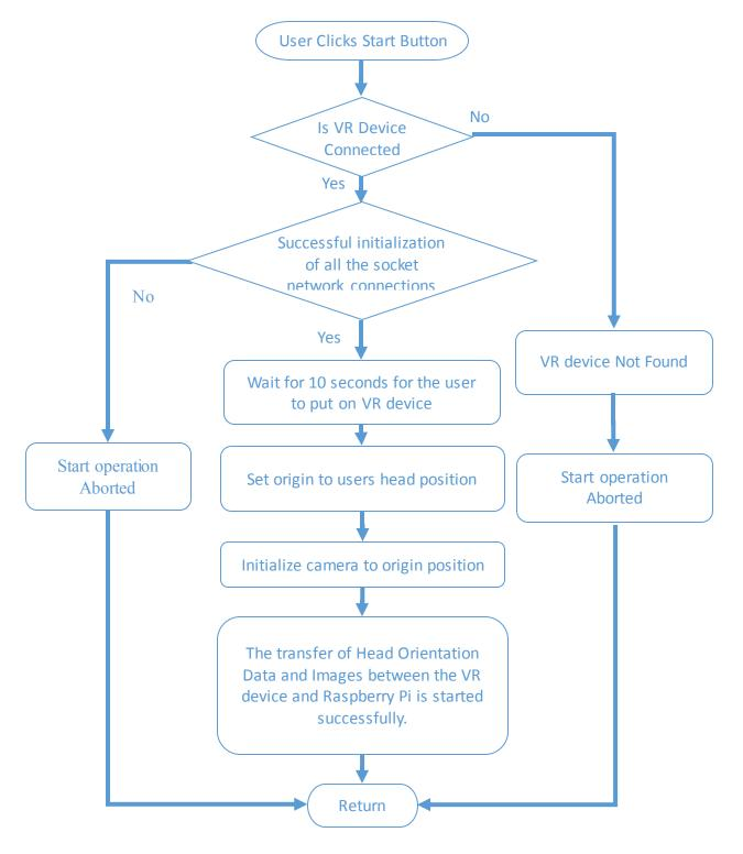
Figure 13: Response of the ART system to the start button
