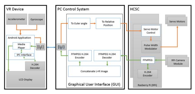
Figure 2: Block level diagram of the ART system
