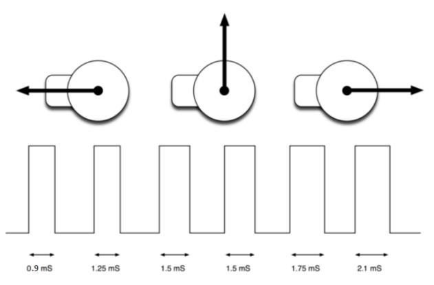
Figure 6: Range of motion of the HS-422 motor [15] [16]
