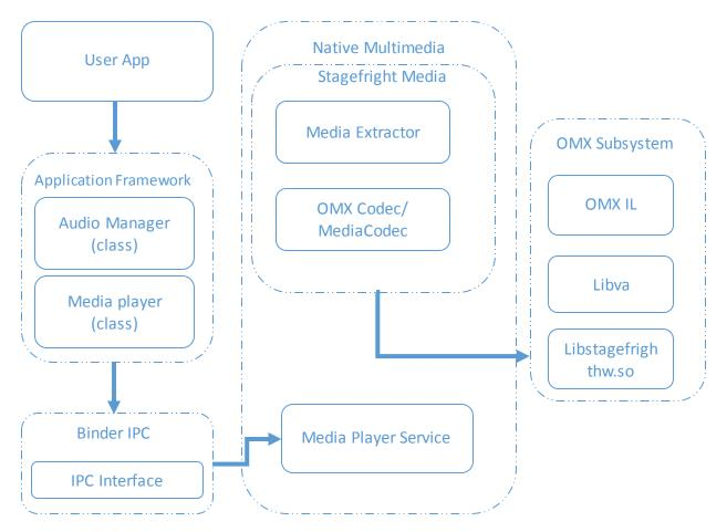
Figure 24: Architecture of Android Media Application
