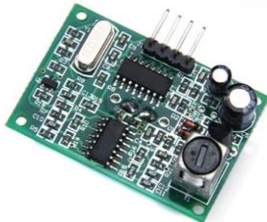
Figure 55: A waterproof ultrasonic distance measuring module for water level monitoring [28]
