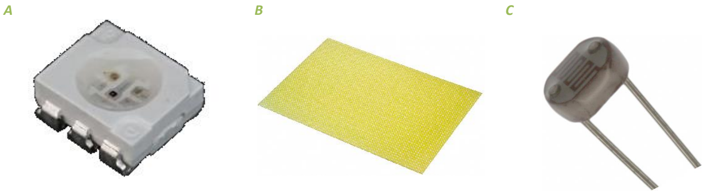
Figure 25: A: The 5050 SMD RGB LED; B: 64P44WE Protoboard; C: The PDV-P8104 Photocell
