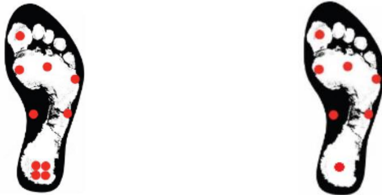
Figure 8: Original design for placement of Force Sensitive Resistors (left) and the revised placement (right)
