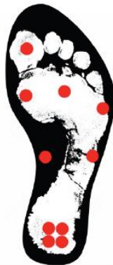
Figure 2: Placement of FSR Sensors under the foot on the insole
