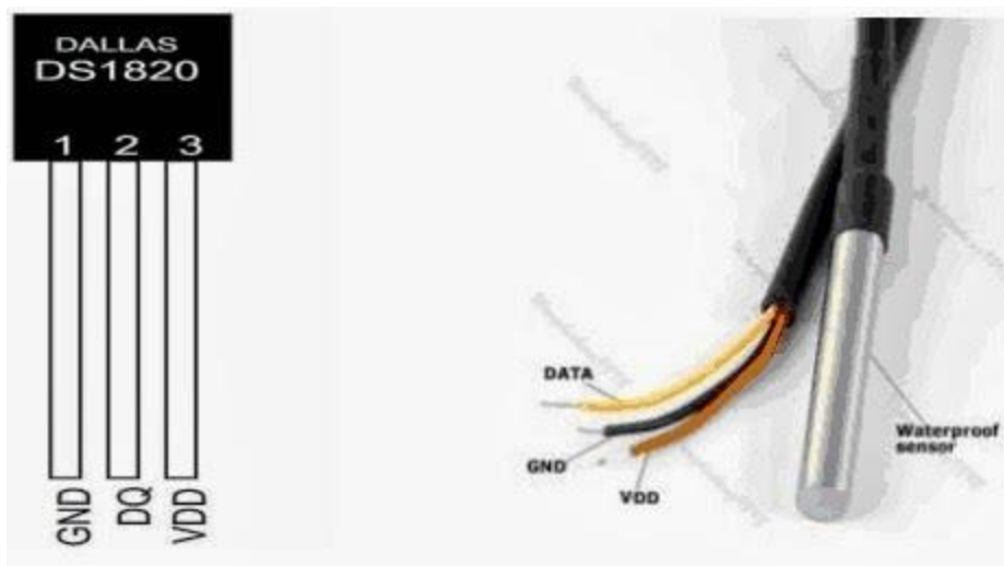
Figure 16:(Left) Pin Assignments for DS1820 temperature sensor; (right) waterproof temprature sensor
