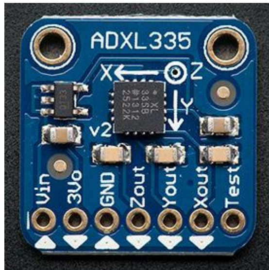
Figure 7: ADXL335: 3-Axis Accelerometer
