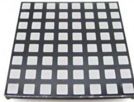
Figure 3: 8x8 RGB LED Matrix
