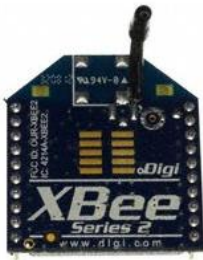
Figure 17: XBee Sender Unit
