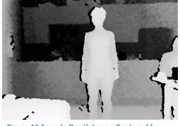
Figure 11 Sample Depth Image Captured by Kinect Depth Camera
