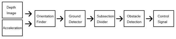
The software package handles the raw data received from the sensors and creates an output control signal to the UI. All processing takes place in the central processor, and the UI commands are passed to the microprocessor, which handles the hardware interfacing through the GPIO pins. Communication amongst processes is taken care of via the Robot Operating System framework and all hardware level communication uses USB connections.
