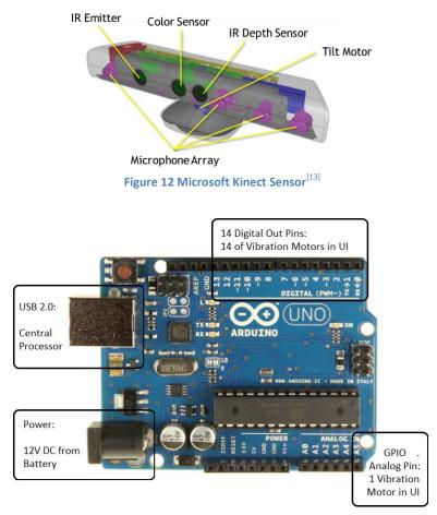
Figure 13 Arduino Uno Microcontroller Board with Planned Connections
