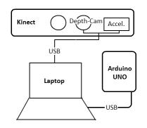
Figure 4 CEHW Overview and Interfacing
