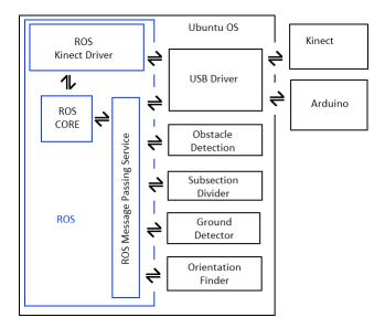
Figure 19 Software Environment Illustration
