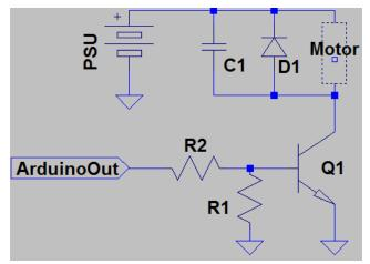
**Figure 16 Vibration Motor Control Circuit**
