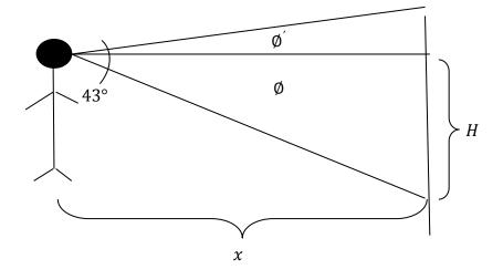
5. Information provided by the accelerometer is in the form of :  $(g_x, g_y, g_z)$ However we do not need to process information in z direction. To obtain information about the angel of the camera in each plane we can use the following relation:
