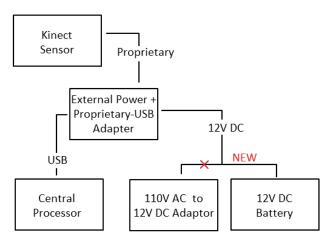
**Figure 5 Kinect Connectivity and Modification**
