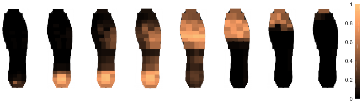
Figure 5: Real-time pressure data generated from the average of six normal steps
