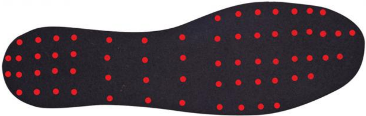
Figure 8: 64 Mapped out Resistors on Insole
