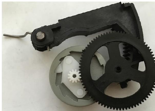
Figure 2: Displays the pedal, gears, and the ratchet.
