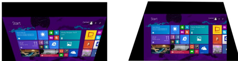
Figure 3 – Perspective correction on original computer screen (left) and the resulting projected screen (right)
