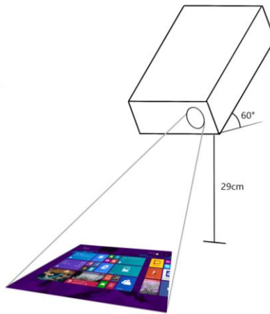
Figure 4 – Sketch of the projector placement and the resulting skewed projection
