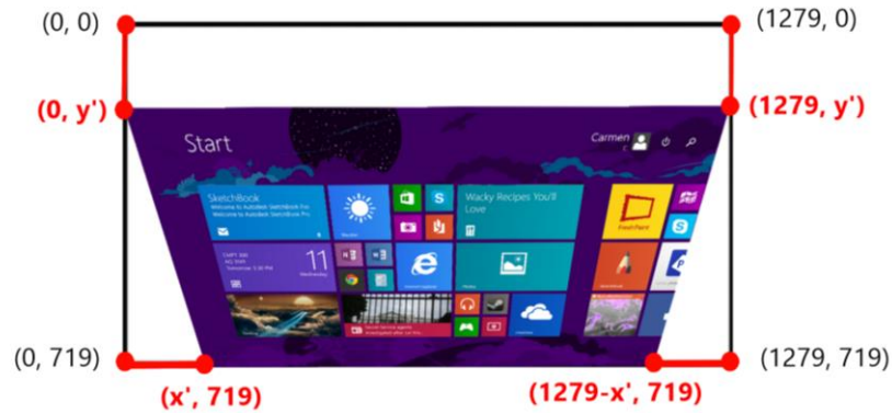
Figure 8 – The four corners of the windows screen and their locations after perspective correction to maximize post-correction screen size
