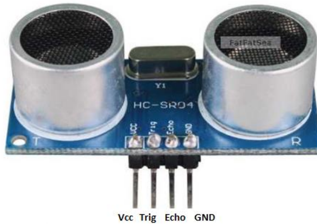
FIGURE 5: HC-SR04 Ultrasonic Sensor [2]
