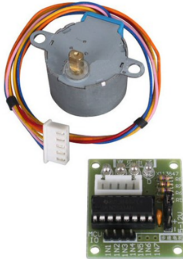
Figure 7: Stepper Motor and Driver [8]
