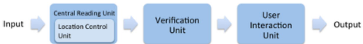
FIGURE 1: LITESPEED GATE SYSTEM HIGH-LEVEL BLOCK DIAGRAM
