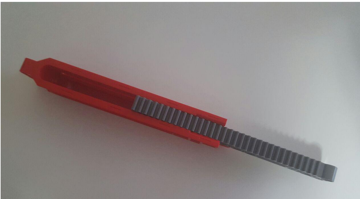
Figure 29: Rack and pinion gears (up view)
