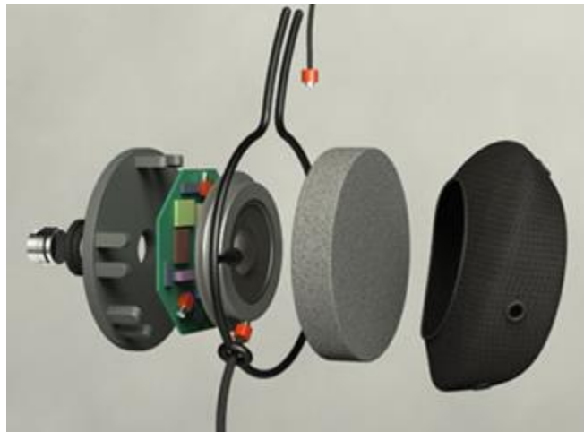
Figure 3: Simple design to allow parts to be replaced [2]
