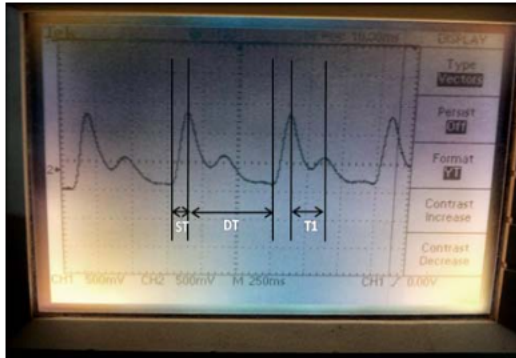
Fig. 2 PPG waveform and its important parameters
