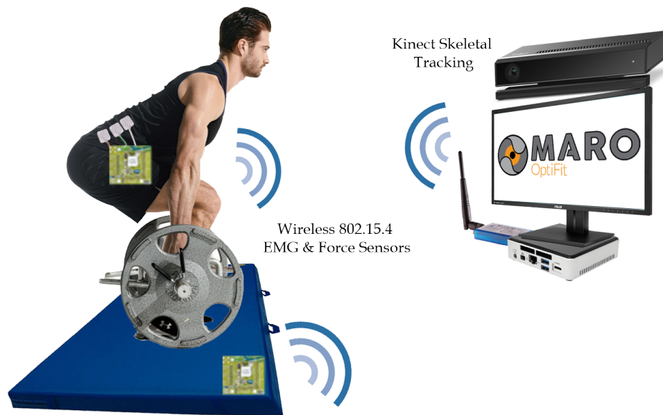
Figure 2: Conceptual design of OptiFit, stock photos courtesy: Men's Fitness, ElectronicSpecifler.com, Microsoft, and StaticWorld.net.
