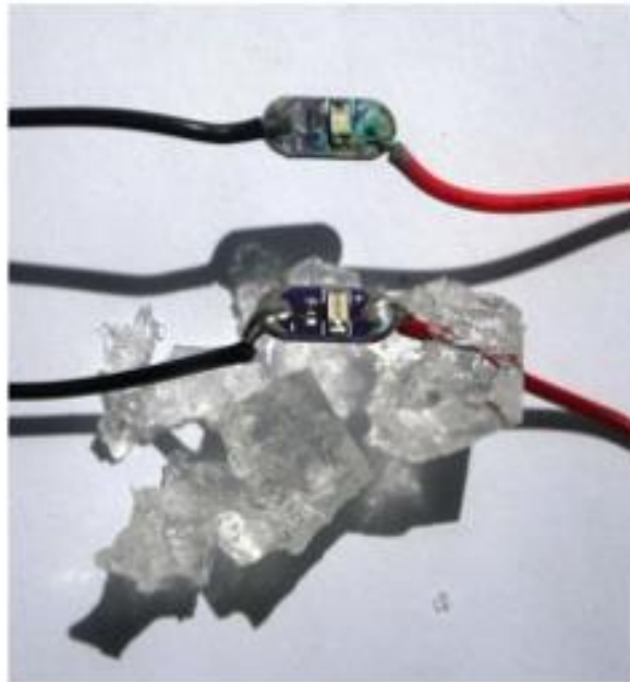
Figure 5 : Unprotected LED versus encapsulated LED [1]
