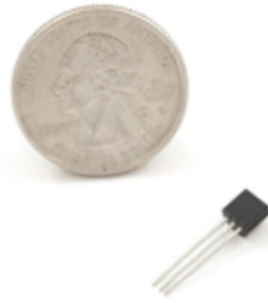
FIGURE 6: SIZE COMPARISON OF THE DS18B20 AND A COIN [7]
