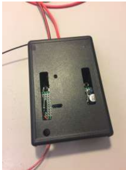
Figure 33: Closed temporary circuit box with vents along bottom of box and output leads out of sides
