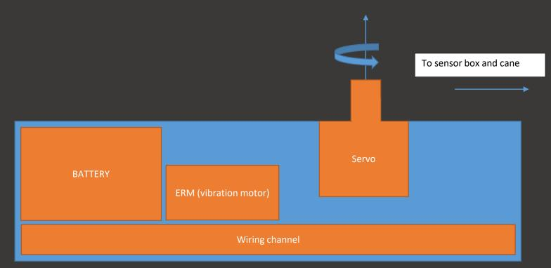
• BATTERY IN HANDLE BUTT AS IT IS HEAVY AND IT MOVES THE CENTER OF GRAVITY AS FUR
