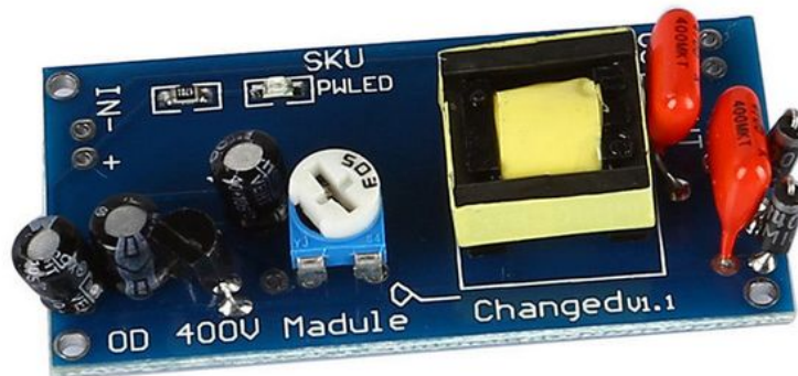
Figure 9. Image of our Ebay boost converter.
