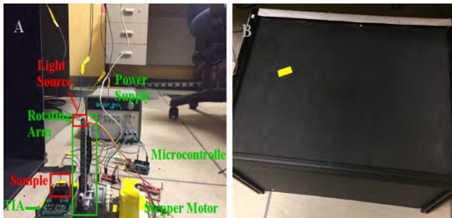
Figure 4-4: Images of the experimental setup. A. The packaged sample is connected via a TIA circuit to the microcontroller (Arduino). The stepper motor is used to rotate the arm holding the light source to several angular positions. The stepper motor is controlled by a microcontroller. B. The system is placed under a black box (Thorlabs) to reduce background lighting [37] ©2017 IEEE.
