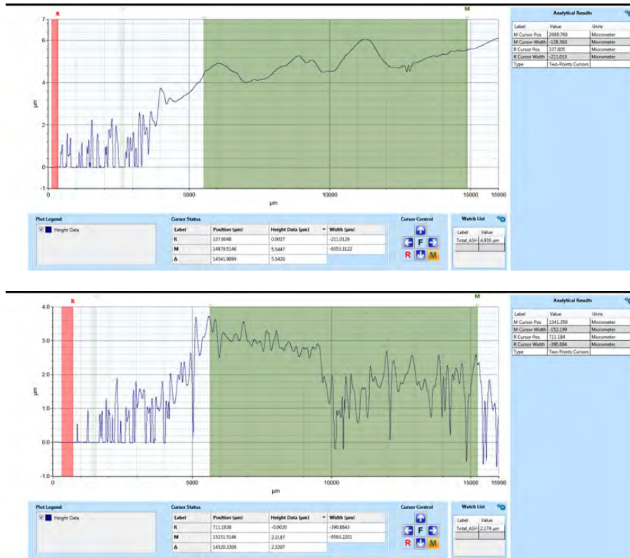
Figure 3-22: Profilemetry results show that resist deposition at 0.3mL/min (top) results in a photoresist thickness of around 5.8\mu\text{m} (not a significant decrease from 0.5mL/min pump flow rate) with a lot of non-uniformity in the deposition. Resist deposition at 0.1mL/min (bottom) results in a photoresist thickness of around 2.1\mu\text{m} (a significant decrease from 0.3mL/min pump flow rate) with a lot of non-uniformity in the deposition with regions of an average thickness of around 3.0\mu\text{m} .
