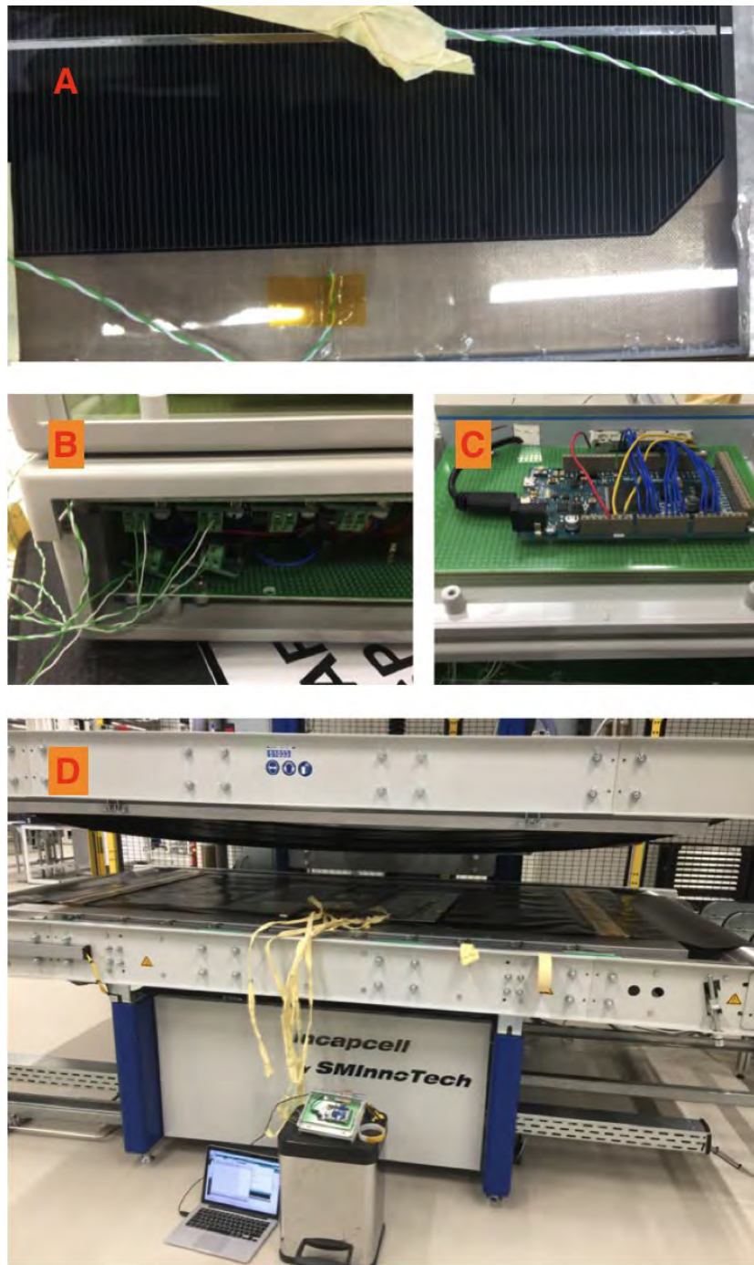
Figure 6-23. Temperature variations studied during the lamination process A. Optical image of thermocouple placed in between TPO-A layers. B,C. Thermocouples are connected to a microcontroller (Arduino Due) to measure temperature readouts during lamination. D Temperature variations readouts are recorded throughout the lamination process.
