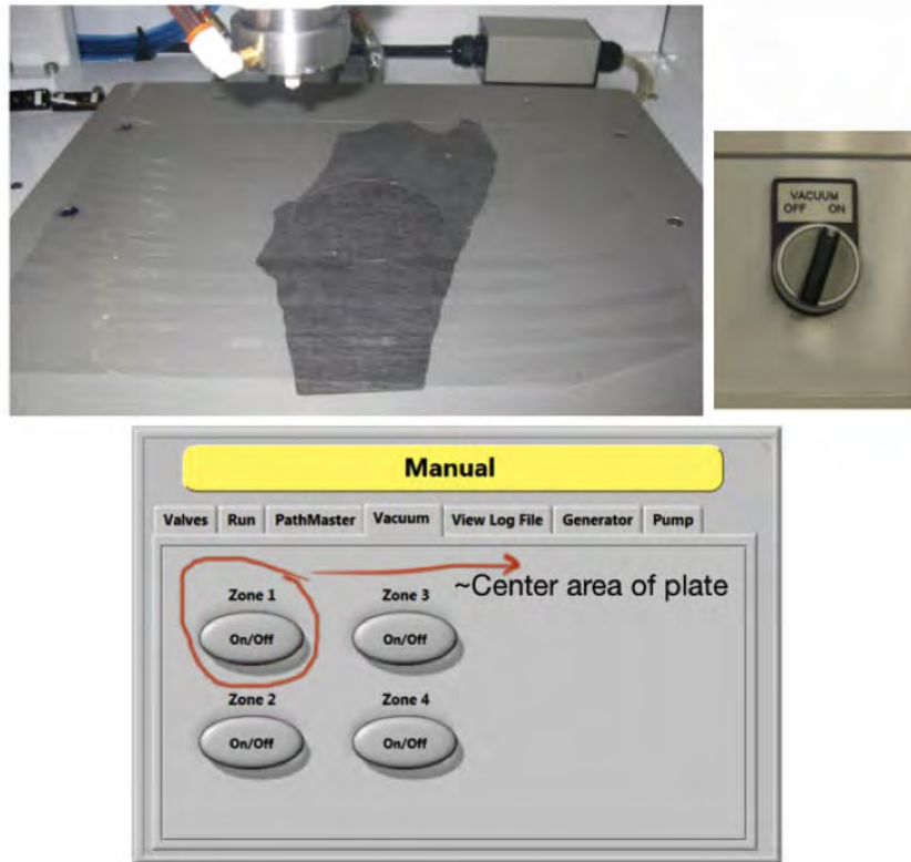
Figure 8-4: The vacuum/hot plate with the vacuum switch and control [87].
