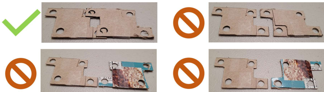
Figure 4.2: Module connector mock-up in all configurations
