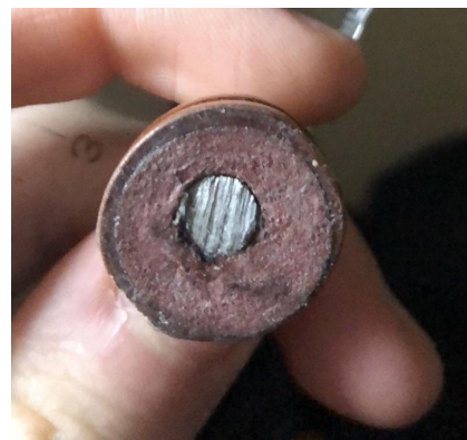
Figure 4.4.4: Metal insert inside chess piece
