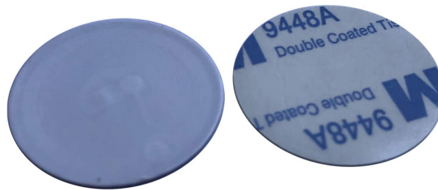
Figure 4.3.4: Anti-metal RFID Tag [16]
