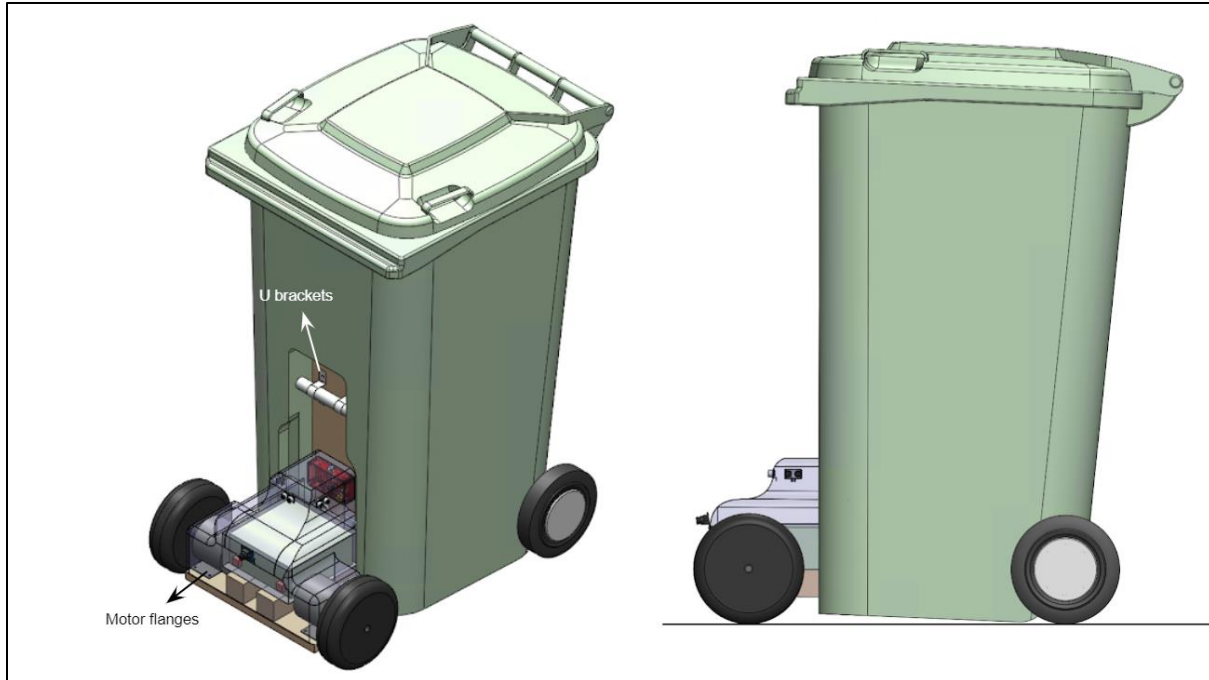
Figure 3. 2: Angled view [left] and side view [right] of Bin Buddy attached to a waste cart
