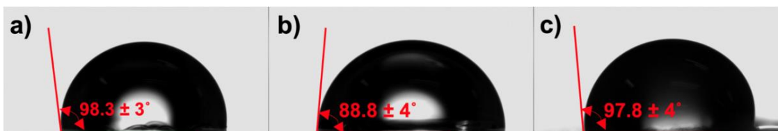
Figure 3-8. Contact angle measurements (10 replicates each) of dry membranes a) N211, b) SPAE, and c) SPPB under at 22 °C and 40% RH.
