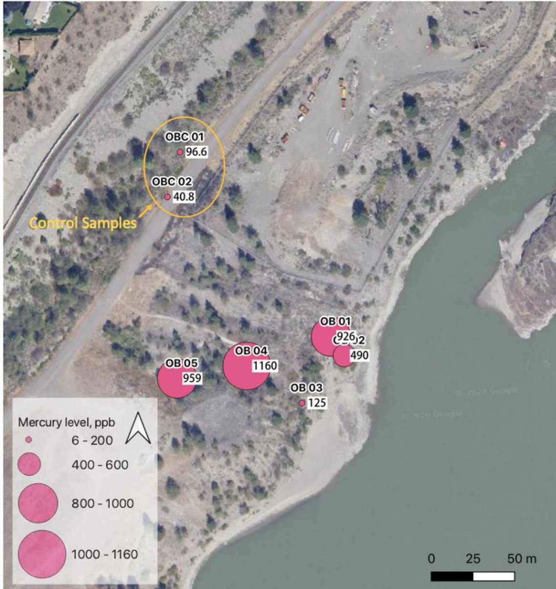
Figure B.1 Sample locations and tHg values in ng/g, equivalent to ppb, for the Lillooet Hydraulic Mining Company site
