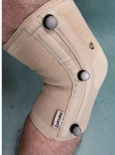
Figure 22 - Reflective marker placement for motion tracking system
