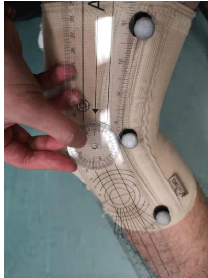
Figure 26 - Calibration process, protractor measuring marker (knee) angle
