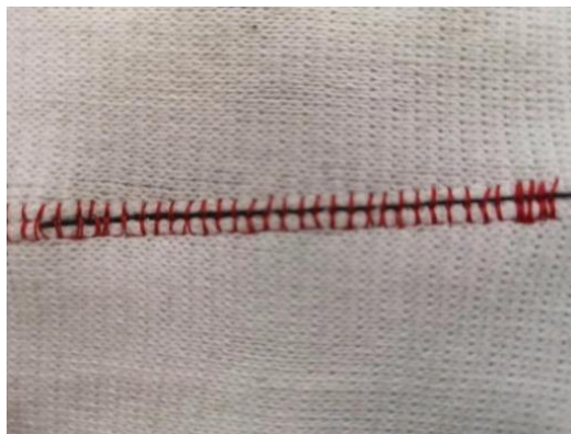
Figure 20 - Sensor embedding by sewing technique to allow stretching
