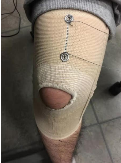
Figure 21 - Sensor embedding through weaving in knee brace with metal snap buttons and conductive thread
