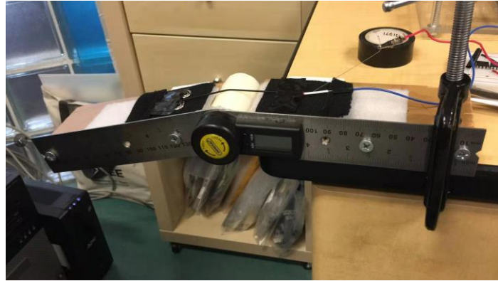
Figure 17 - Bending stage test setup
