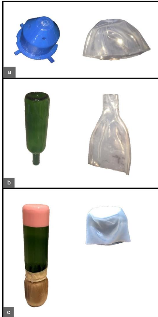
Figure 3.32: Different Silicone mold iteration. Silicone was applied using a brush in these molds.
