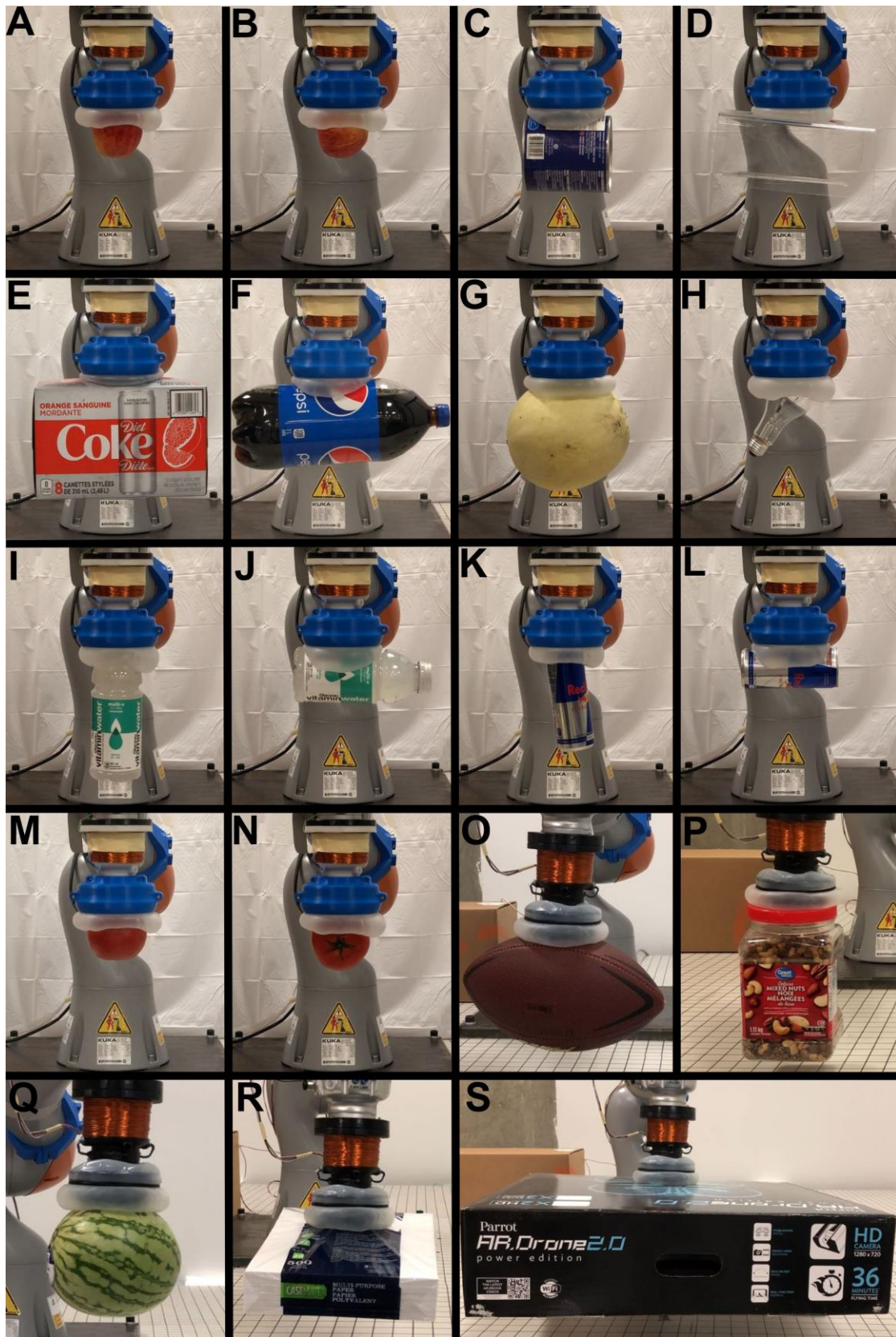
Figure 4.7: Picking up objects with various shapes and weights.
