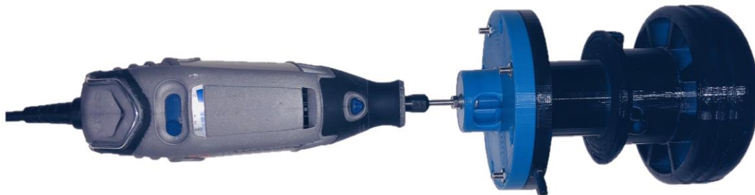
Figure 3.8: Gripper's body attached to a rotary tool for wrapping the coil
