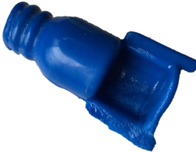
Figure 3.11: Overexposure of an ABS part to acetone vapor
