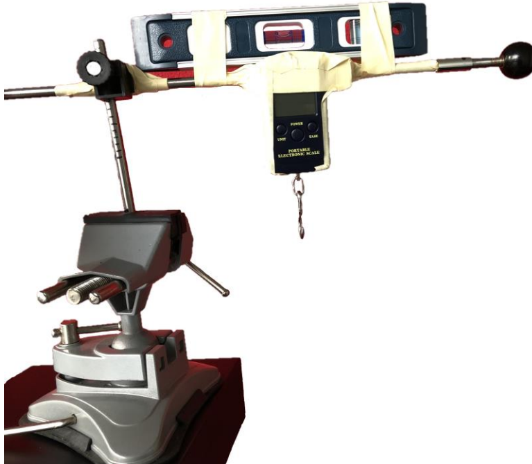
Figure 3.14: Force sensor attached to a leveling device
