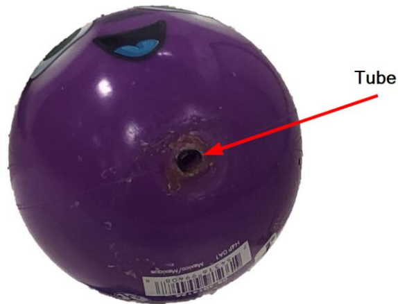
Figure 4.3: A rubber ball with a tube inserted to create a hole
