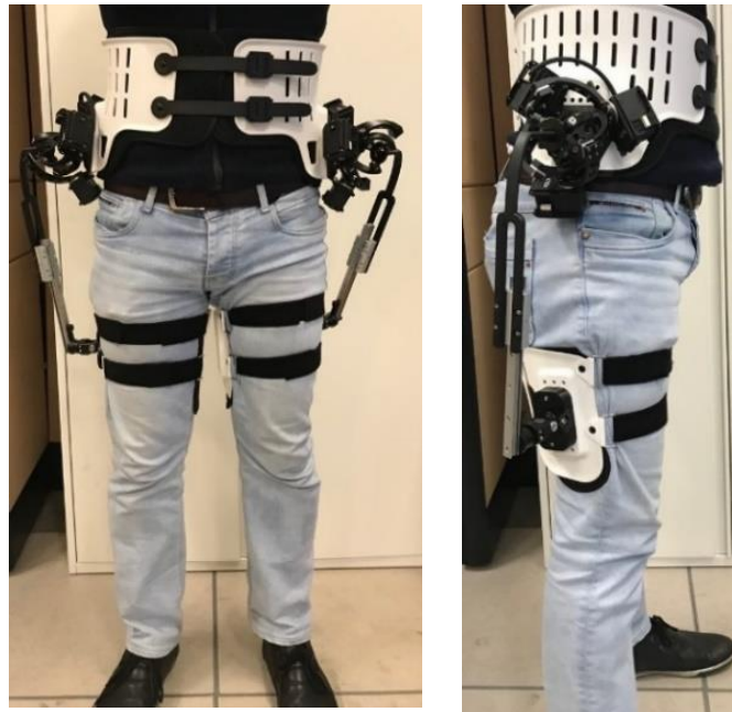
Figure 1.10: Hip exoskeleton robot with agile eye mechanism
