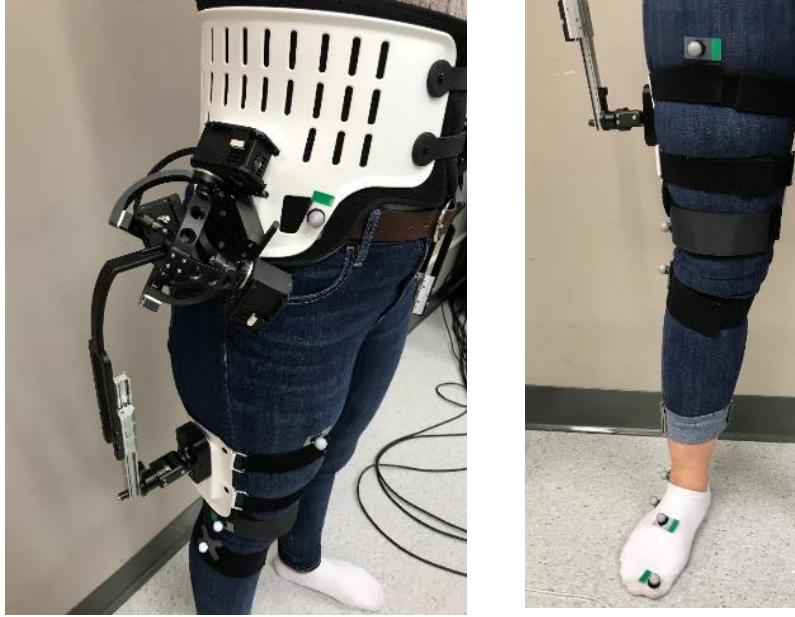
Figure 3.2. Optical markers placements while wearing the hip exoskeleton
