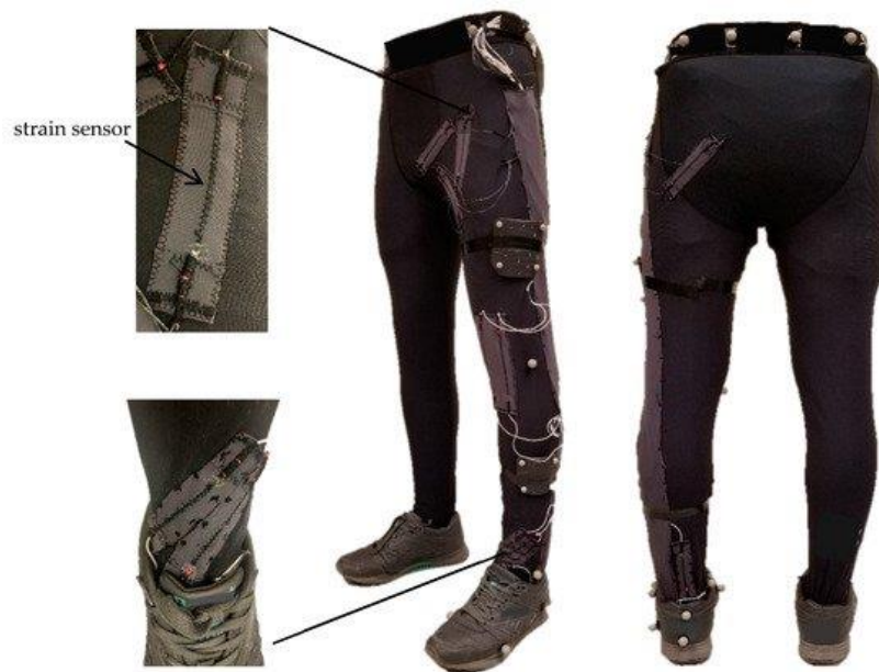
Figure 2.1 Example of a smart garment with resistive strain sensors [48]. This image is licensed under a Creative Commons Attribution license (CC BY). Source image: Gholami, M.; Rezaei, A.; Cuthbert, T.J.; Napier, C.; Menon, C. Lower Body Kinematics Monitoring in Running Using Fabric-Based Wearable Sensors and Deep Convolutional Neural Networks. Sensors 2019, 19 , 5325, https://www.mdpi.com/1424-8220/19/23/5325 . Accessed on 20/September/2020.
