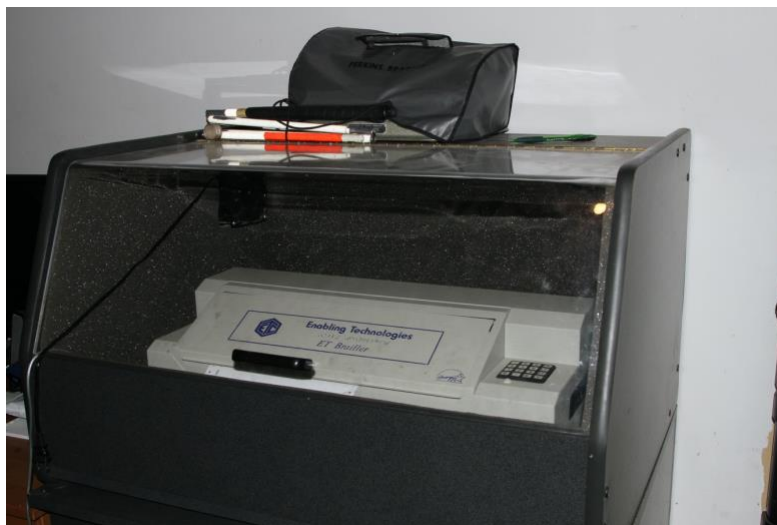
Figure 4.2. A large brailer at a participant's home, which is used to print paper documents in braille
