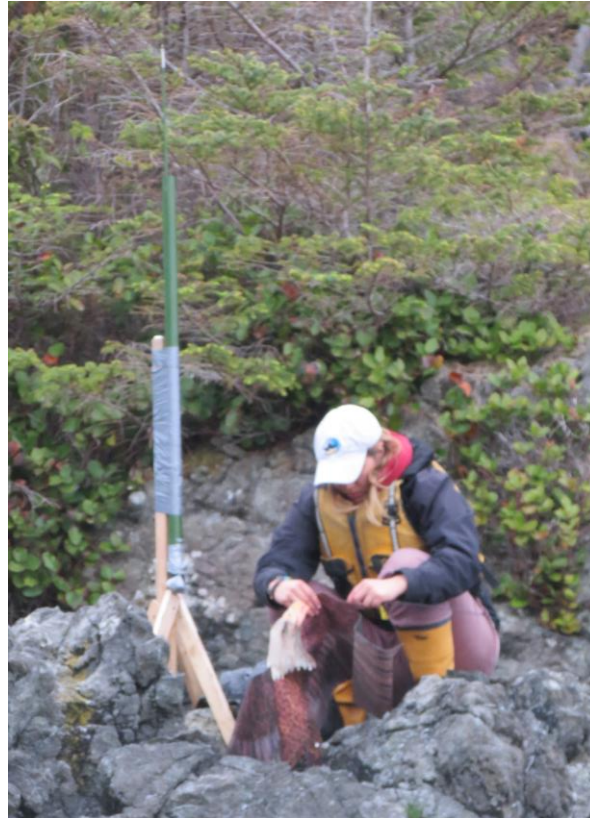
Figure C1 Kite Stand with attached fibreglass extendable pole, researcher unpacking kite to attach to stand.
