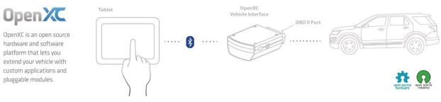
Figure 3-2: OpenXC Hardware and Software Platform
