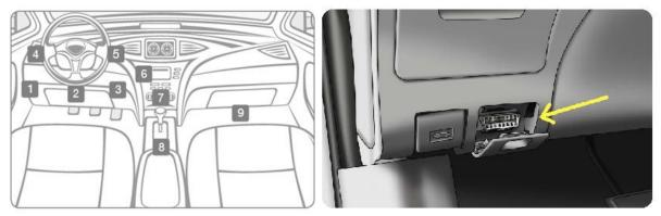
Figure 2-2: Example of a OBD-II Diagnostic Port Location
