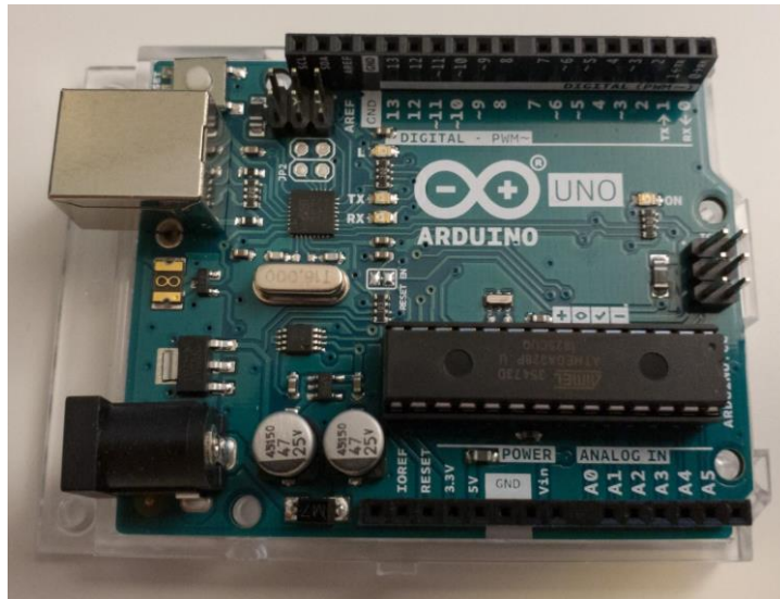
Figure 2-4: Arduino Uno and top female connectors
