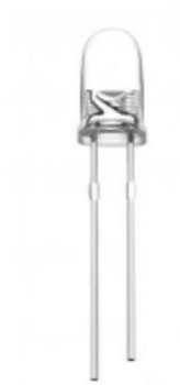
Figure B.3.1.1: (a) Momentary Switch with 3V LED (b) 3V Red LED
