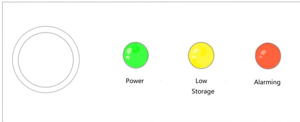
Figure B3.6.2: Front Panel (Left to Right: Self-Checking Button with White LED, Green Power LED, Yellow Low Storage LED, Red Alarming LED)
