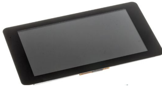
Figure 10: 7" Multi Touch LCD screen[5]
