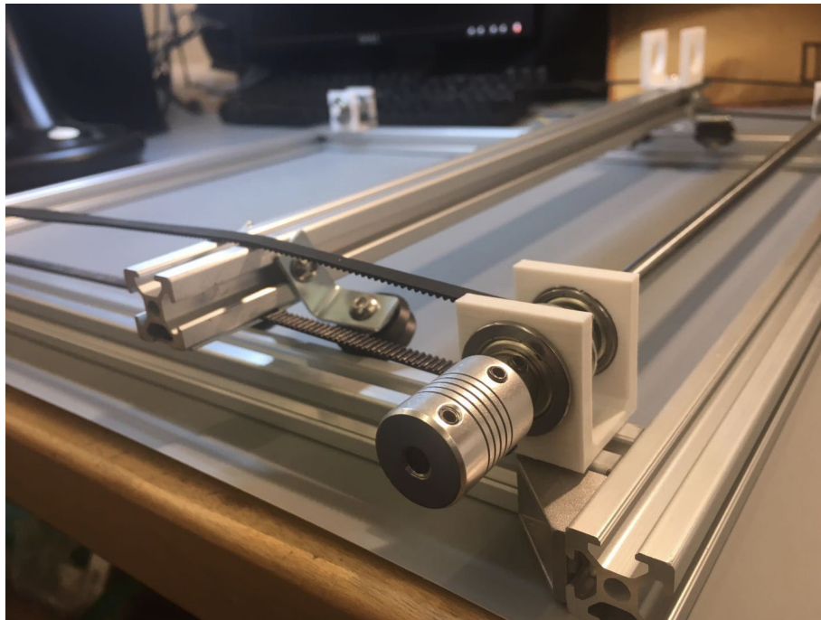
Figure 4.0 X-Y table Design
