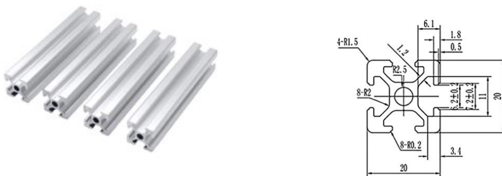
Figure 4.1b Aluminum Extrusion Specification [5]
