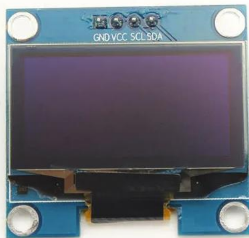
Figure 27: Four pin I2C 1.3" 128x64 OLED. Found at Ref. [17]. However, many other modules exist on the market.
